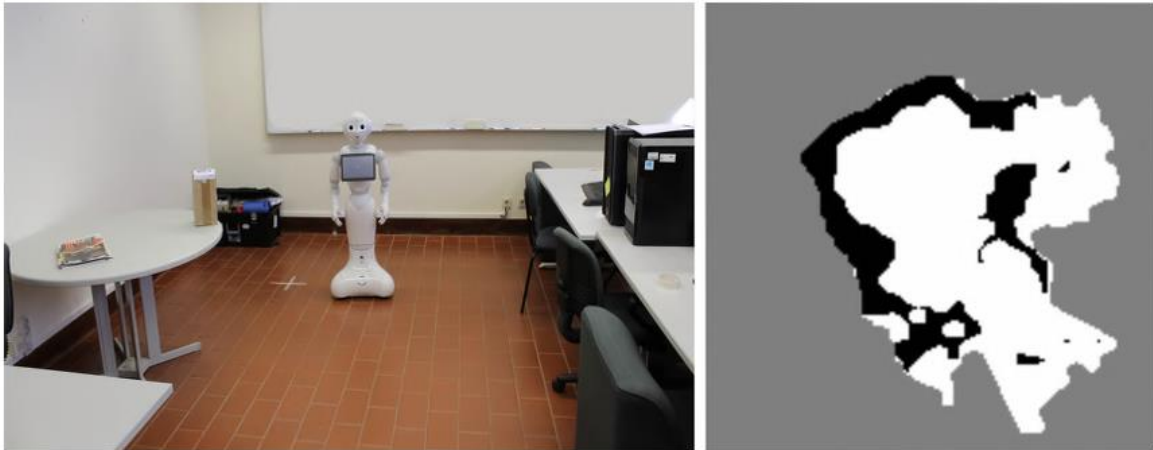
Figure 28 - Pepper mapping environment, real environment (left) and represented map (right).
