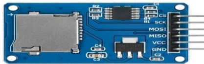
Figure 2-18. SD Card Module [36]
