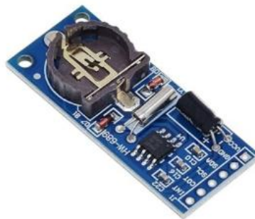
Figure 2-17. RTC PCF85 Module[61]
