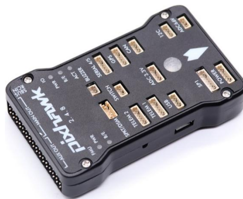
Figure 40 Pixhawk 2.4.8 Flight Controller
